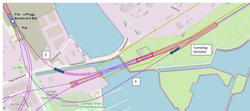
Figure 30 - TBM launch location (Blue arrows)- Red outline is the Øresund metro ramp structure.
