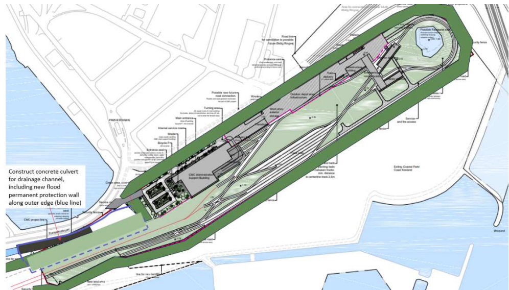
Figure 38 - Phase 4 - Øresund metro Ramp Construction Sequence.
