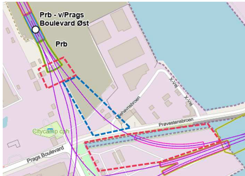
Figure 29 - Possible Worksite Areas to be safeguarded for construction of tunnels and TBM removal during construction of Øresund metro.
