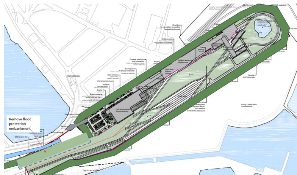
Figure 37- Phase 3 - Øresund metro Ramp Construction Sequence.
