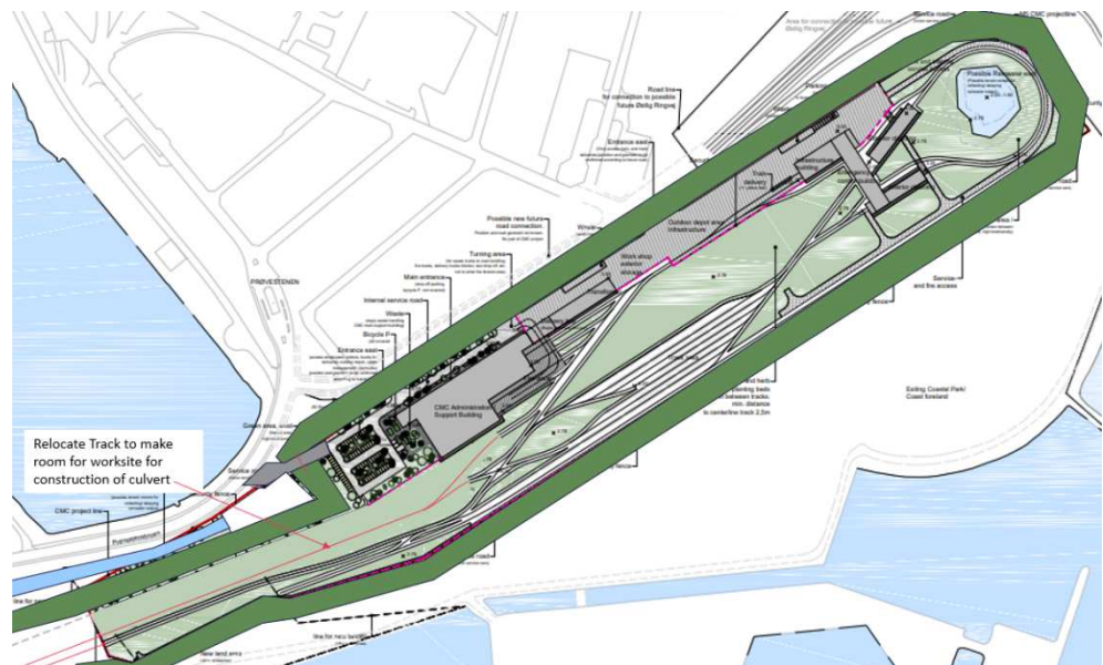
Figure 35 - Phase 1 - Øresund metro Ramp Construction Sequence.
