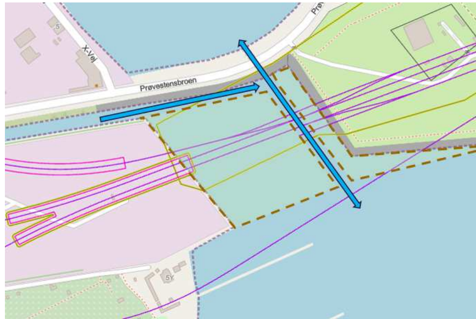
Figure 3 Culvert and drainage constraints (Culvert and drain channel shown as blue arrows, reclaimed land shown as brown dotted line)
